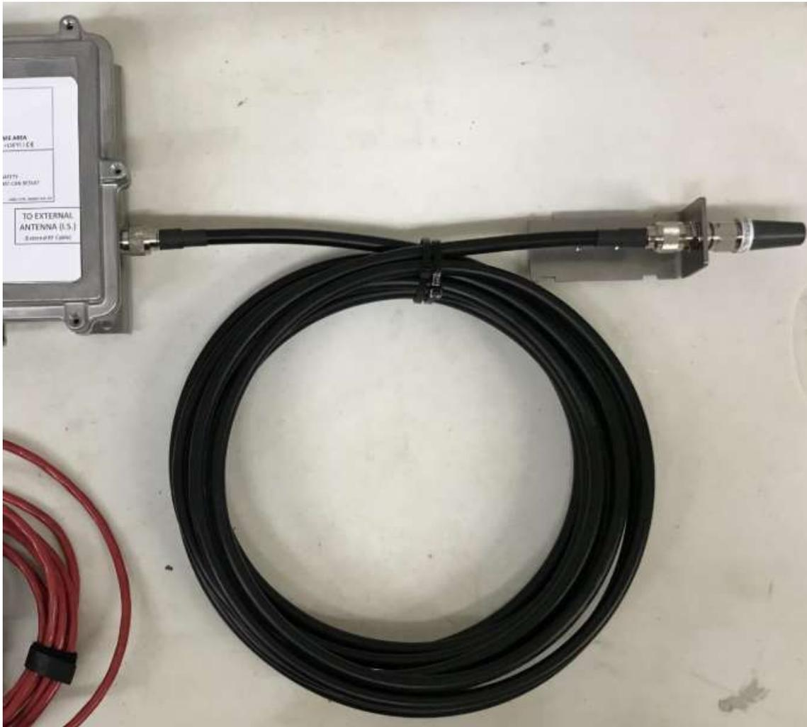
Figure 3: External antenna assembly connection
