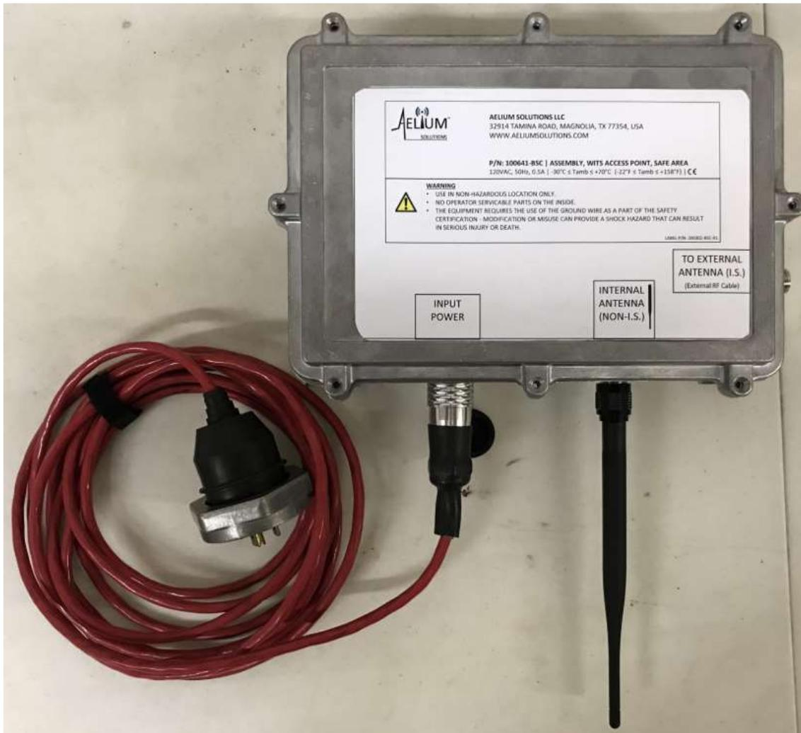
Figure 2: Internal antenna connection – safe area use only
